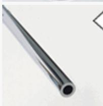
High stress resistance machine-trued hollow steel bars - diameter 16mm - coated with anti-rust chromium-plating - The quality of the materials used adds to the thickness of 2,2mm to prevent the bars from bending, maintaining a perfect shape for a long time. On choice going-through (also called solid) bars or telescopic bars.
